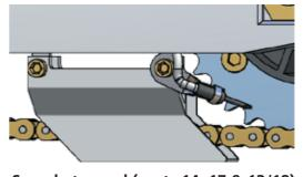
Use adhesive clips (part 8) and cable ties (part 12) to route tubing dispenser assembly (part 14) to REP location. Hint: Use IPA Wipe (part 9) to degrease surfaces before adhering.
