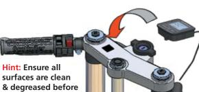
**Bracket Mount.** Fits to any existing M5/M6 bolt. Fit display unit to bracket (part 5) using M3 screws (part 16).
